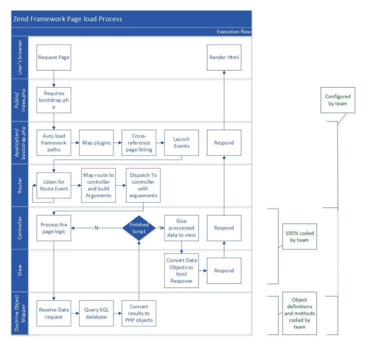
This diagram describes the top level execution flow for the PHP framework. To describe the process simply: ZF2 uses a combination of autoloaders and event driven managers that route to Controllers, which in turn process user input, and eventually return html via view files.
